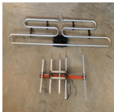
Figure 4. Typical television antenna (Yagi-Uda).
